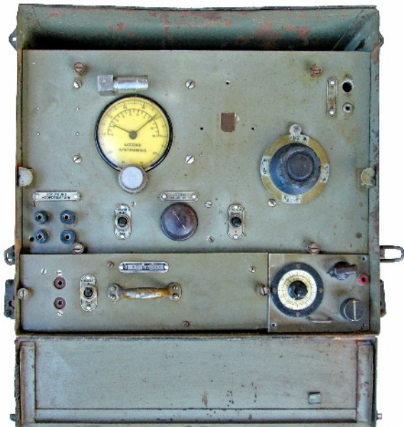
Front panel view of RP 39 and associated 6V power unit in its metal enclosure. The controls fitted on the (probably not original) panel of the right hand side of the power unit were a later addition.
