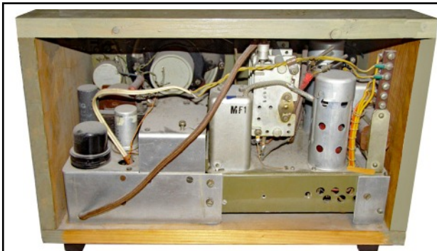
Retrieved from the Internet were two photos of a (probably converted to medium wave) receiver built with salvaged parts of the Belgian RP 39 receiver. The rotary coil block was removed, a single range (believed medium wave broadcast band) coil block and an AC Mains power unit fitted in its place. The wooden case and front panel were painted olive drab, a loudspeaker was fitted on the place of the former range switch and a test meter mounted in the front panel.
