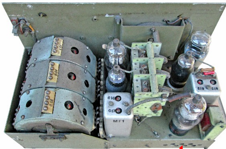
The photo above shows the top side of the chassis with a massive rotary coil block at the left, believed to be a separate assembly. Sockets slid into a 6-pin contact block fitted in the case.
