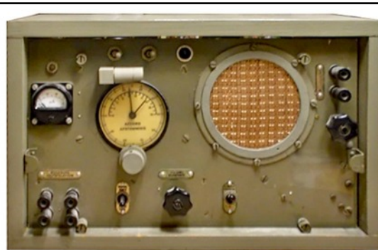
Retrieved from the Internet were two photos of a (probably converted to medium wave) receiver built with salvaged parts of the Belgian RP 39 receiver. The rotary coil block was removed, a single range (believed medium wave broadcast band) coil block and an AC Mains power unit fitted in its place. The wooden case and front panel were painted olive drab, a loudspeaker was fitted on the place of the former range switch and a test meter mounted in the front panel.
